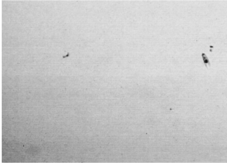
Fig. 2.13 Nomarski micrograph of MBE#2511 (0.64 \mu\text{m} InGaAs layer nominally lattice matched to InP).
